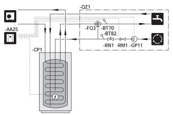
OUTLINE DIAGRAM WITH ADDITIONAL WATER HEATER, HWC AND ELECTRONIC MIXING VALVE
